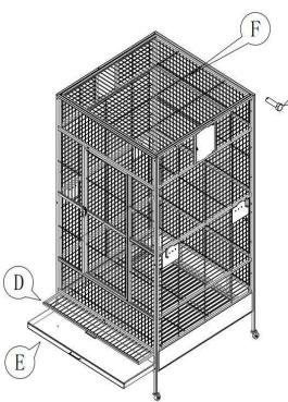
**Step 3:** Put D and E in the corresponding slideways, put F on the top of the top module, and fix it with screws K.
