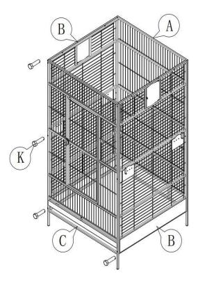
**Step 1:** Connect A,B,C with screws K and fix them as the sequence shown in the picture.
