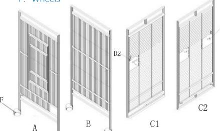
Step 1: Assemble the cup holder D2 on the door of C1 and C2, use screws M3 to screw them together. Then put D1 on D2, put the wheel F into the legs of A and B. See the picture on left.
