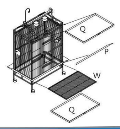
**Step 5:** Assemble P around the cage, use M3 and N to fix them. Assemble Q and W as the arrows indicate, see the picture on left, put L1 inside the cage body. The cage is finished!
