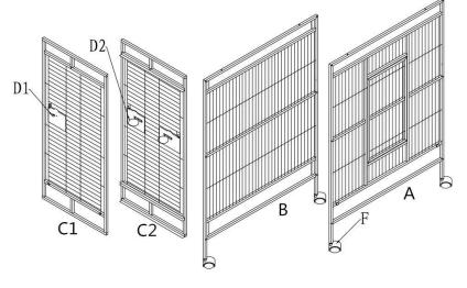
**Step 1:** Use M3 to fix D2 onto doors of C1 and C2. Assemble D1 in the middle of D2. Put F into the legs on A and B, see the picture on left.
