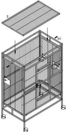
**Step 3:** Put E on the top, and use M4 to fix it, see the picture on left.
